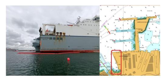
As a precautionary measure, Oil Spill Boom has been deployed around the stern of a Casualty vessel berthed on County Wharf.
